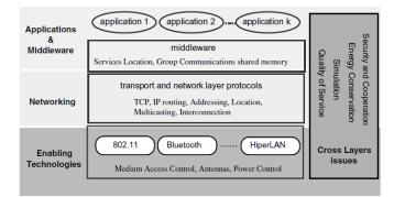
Fig. 1. A simple MANET architecture
